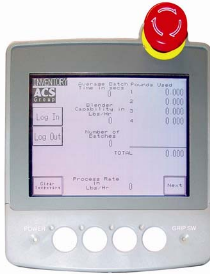
Figure 9: Typical Mitsubishi Controller Touch Screen Display
